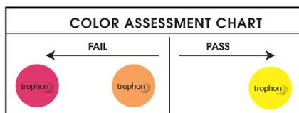
Disc impregnated with a dye that turns from red to a signal yellow to visually indicate the successful completion of a disinfectant cycle. Complements the patent pending automated sensors that are internal to the Trophon EPR® and also signal successful disinfection. The indicator is used each cycle and provides an annuity revenue stream.
